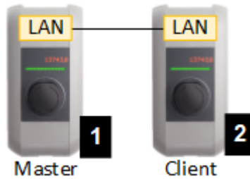
Fig. 2-3: Direct connection of master and client
